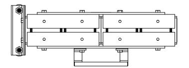
Capacity: 12 Tons Each Roller Material: Steel
