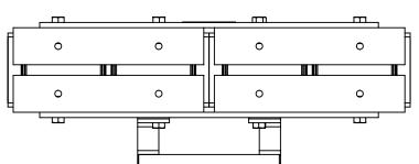
Capacity: 12 Tons Each Roller Material: Steel Weight: 43 lbs.
