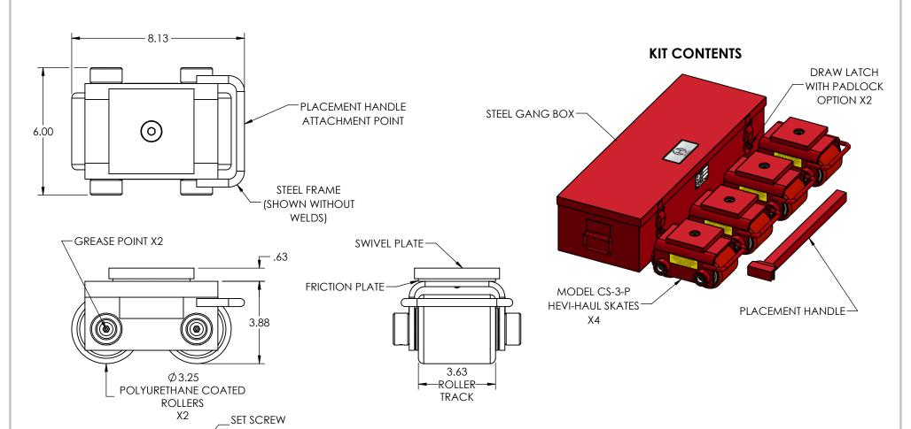
Capacity: 6 Ton Kit, 1.5 Ton Per Skate Roller Material: Polyurethane Coated Weight: 103 lbs.
