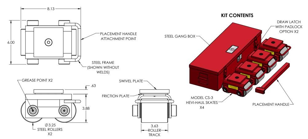
Capacity: 6 Ton Kit, 1.5 Ton Per Skate Roller Material: Steel Weight: 127 lbs.
