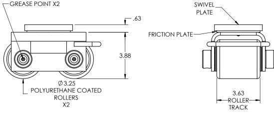
**Capacity:** 1.5 Tons Each **Roller Material:** Polyurethane Coated
