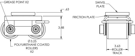
**Capacity:** 2.5 Tons Each **Roller Material:** Polyurethane Coated
