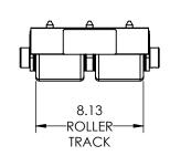
Capacity: 10 Tons Each Roller Material: Polyurethane Coated Weight: 81 lbs.
