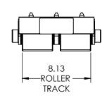
**Capacity:** 10 Tons Each **Roller Material:** Steel
