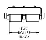
Capacity: 20 Tons Each Roller Material: Polyurethane Coated Weight: 111 lbs. Colorway: Hevi-Haul Red Country of Origin: United States of
