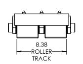
Capacity: 25 Tons Each Roller Material: Steel
