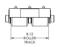
**Capacity:** 6 Tons Each **Roller Material:** Polyurethane Coated
