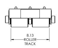
Capacity: 6 Tons Each Roller Material: Steel Weight: 58 lbs.
