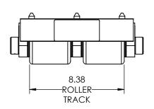
Capacity: 20 Tons Each Roller Material: Polyurethane Coated Weight: 69 lbs. Colorway: Hevi-Haul Red Country of Origin: United States of
