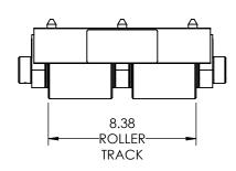
Capacity: 20 Tons Each Roller Material: Steel Weight: 81 lbs.
