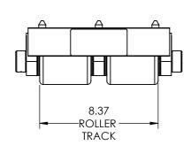
**Capacity:** 30 Tons Each **Roller Material:** Polyurethane Coated
