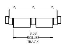
Capacity: 30 Tons Each Roller Material: Steel Weight: 104 lbs.
