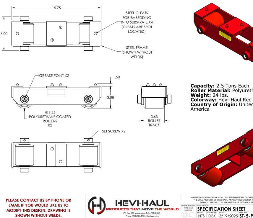
Capacity: 2.5 Tons Each Roller Material: Polyurethane Coated Weight: 24 lbs. Colorway: Hevi-Haul Red Country of Origin: United States of
