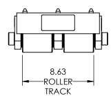
**Capacity:** 100 Tons Each **Roller Material:** Steel
