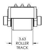
**Capacity:** 7.5 Tons Each **Roller Material:** Polyurethane Coated
