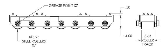
Capacity: 12.5 Tons Each Roller Material: Steel Weight: 121 lbs. Colorway: Hevi-Haul Red Country of Origin: United States of America
