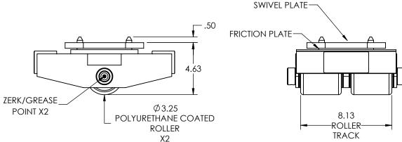
Capacity: 3 Tons Each Roller Material: Polyurethane Coated
