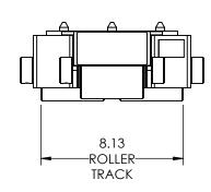
Capacity: 4 Tons Each Roller Material: Steel
