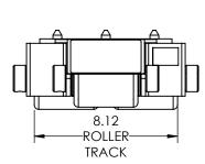
Capacity: 7.5 Tons Each Roller Material: Polyurethane Coated Weight: 58 lbs. Colorway: Hevi-Haul Red Country of Origin: United States of
