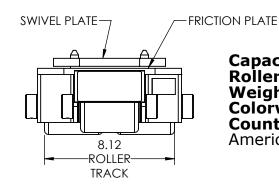
Capacity: 4 Tons Each Roller Material: Steel
