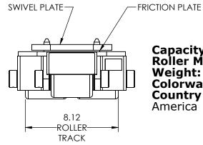
**Capacity:** 10 Tons Each **Roller Material:** Polyurethane Coated
