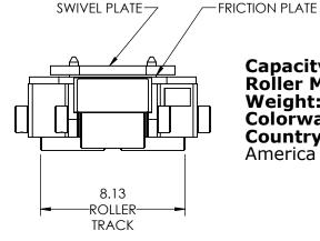
**Capacity:** 10 Tons Each **Roller Material:** Steel
