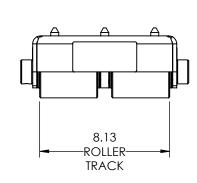
Capacity: 15 Tons Each Roller Material: Steel Weight: 63 lbs.
